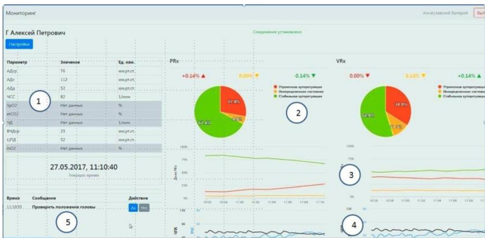
Figure 4. ICPCDS system’s Web interface. 1 – Digital table of monitoring parameters. 2 – Autoregulation indices PRx and VRx presented as “living” circular diagrams updated every five seconds; the green sector expresses good cerebral autoregulation, the red sector marks the zone of lost autoregulation, the yellow sector is the zone of uncertainty. 3 – Linear graphical trends of circular diagram sectors. 4 – Synchronized trends of ICP CPP charts. 5 – Window for displaying messages from the step protocol of the Arden Syntax CDS system.
