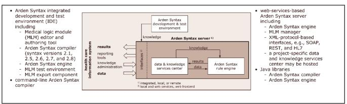
Figure 1: Suite of Arden Syntax software—service-oriented architecture and software components
